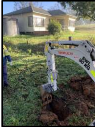
Image 1: This image depicts the location of Pit 12, south of the onsite residential dwelling. In this area, near the highest point of the property, the soil consisted largely of organic fill material, with some sandstone boulders also being encountered.
